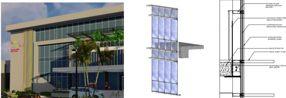
**Gambar 4. Detail Curtain Wall**
