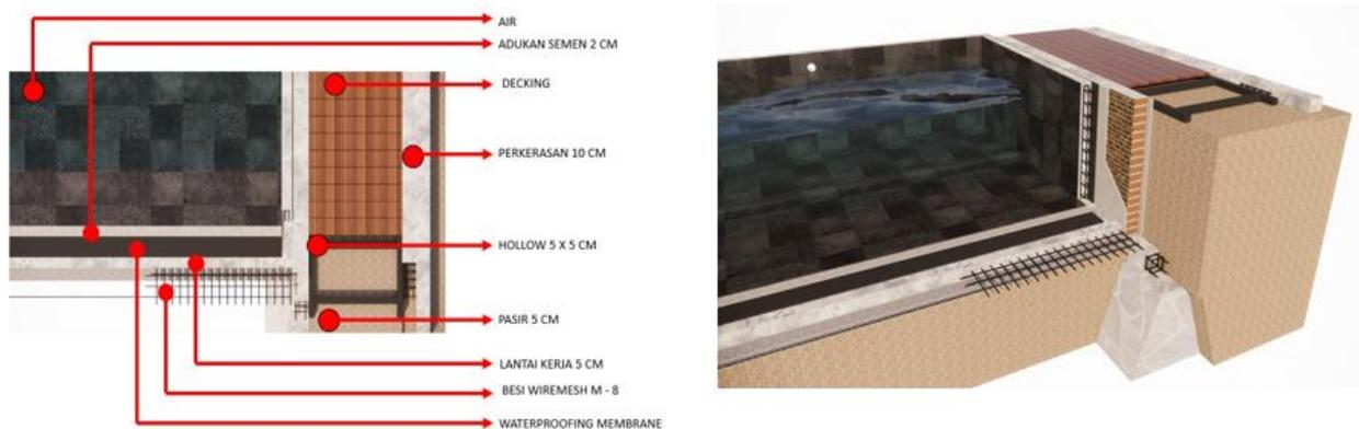
**Gambar 3.4.2 Detail Kolam / Cooling Effect**
