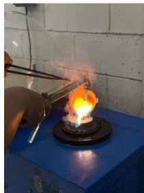
Gambar 16. Proses pengecoran limbah logam kuning.
