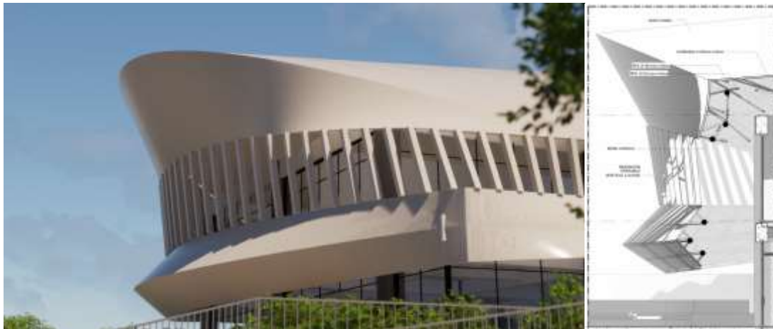
Gambar 6. Detail Automated Vertical Louvre Shading system Sumber : Pribadi
