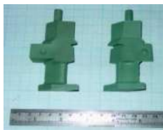
Fig. 3: Wax pattern of the injection results
