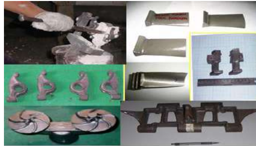
Fig. 5: Casting product results by using investment casting
