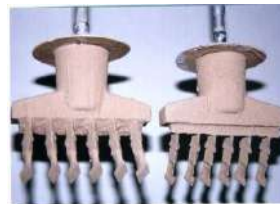
Fig. 4: Ceramic slurry made of domestic zircon sand
