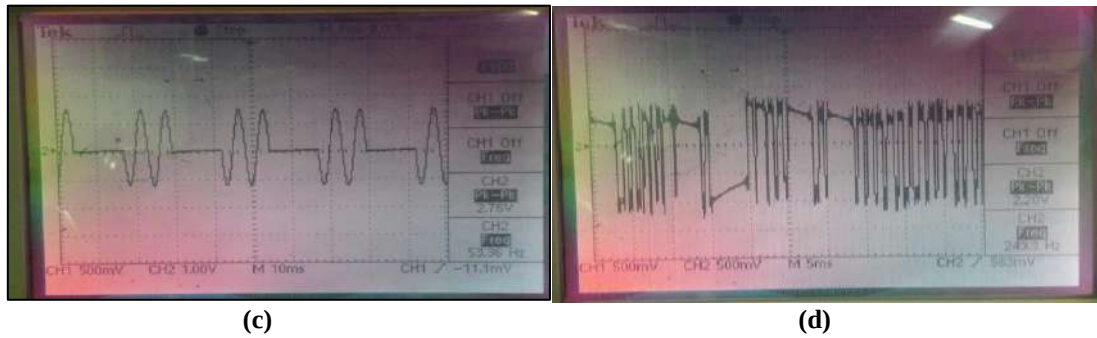
Fig.7 : Output Signal System ASK (a) m-file (b) Simulink (c) Implementation of Modulator output Signal (d) Implementation Signal after Demodulation
