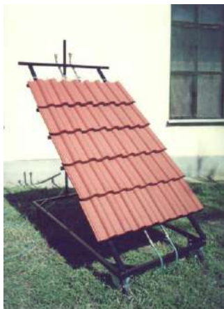
Fig. 4: The layout of a shell-structured solar collector
