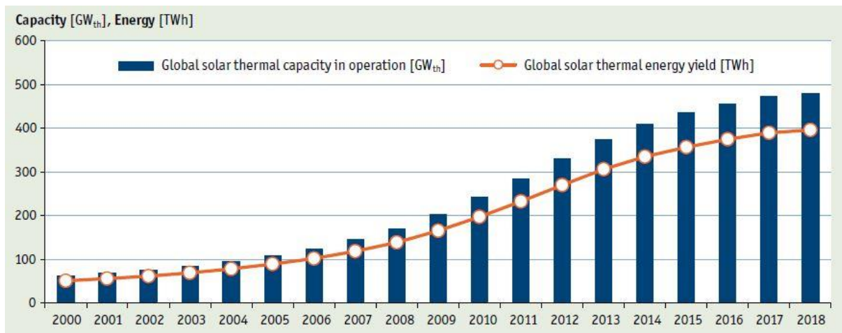
Fig. 2: Global solar thermal capacity in operation and energy yield for the period of 2000-2018
