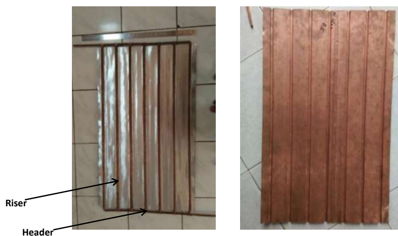
Fig. 1: The tested solar collectors with (a) aluminum absorber plate (b) copper absorber plate
