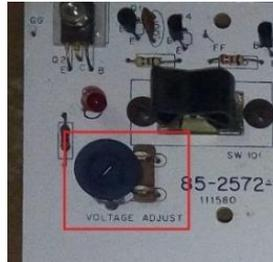
Gambar 3.3. Resistor *variable*
