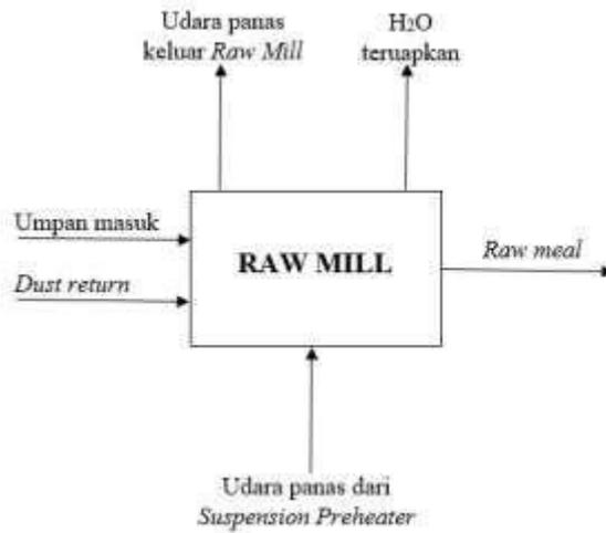
**Gambar 1. Diagram Alir Raw Mill**
