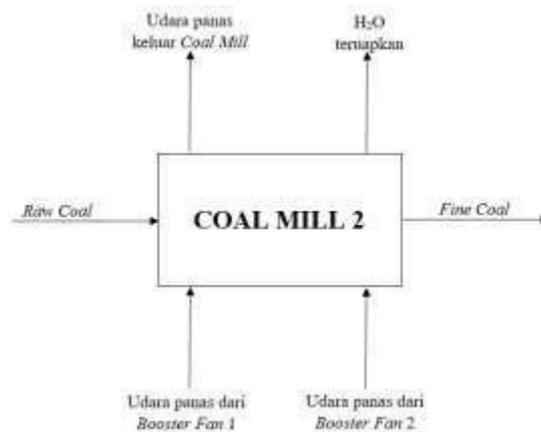
**Gambar 3. Diagram Neraca Massa Coal Mill 2**
