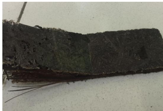
Gambar 7. Fenomena Patahan Uji Bending
