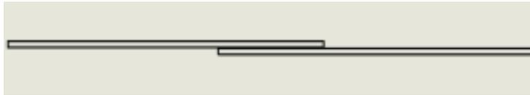
**Gambar 3.2 Jenis sambungan single lap joint**
