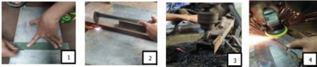
Gambar 8. Langkah-langkah proses pembuatan spesimen single lap joint
