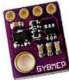
Gambar 4. Sensor bme280 ( Sumber: (Sari et al., 2020).
