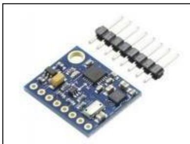
**Gambar 3. Sensor Imu ( Sumber:(Mudarris & Zain, 2020).**
