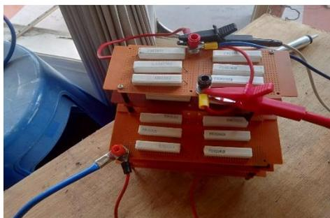
Gambar 3. Voltage Devider
