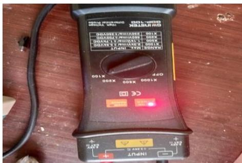
Gambar 5. Deferential Probe
