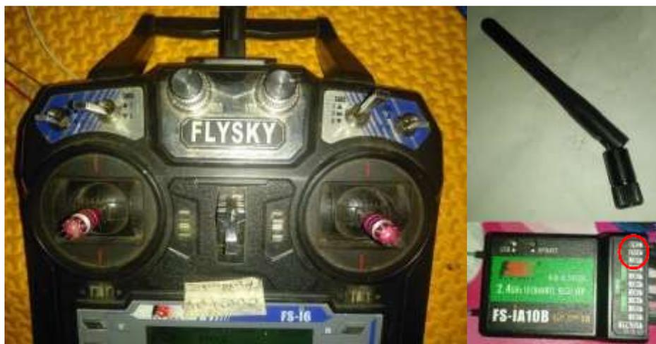
**Gambar 5. Remote control, transmitter dan receiver**
