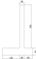
Gambar 3. Dimensi Dinding penahan Tanah
