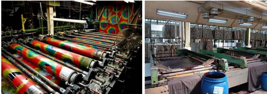
**Gambar 1. Jenis *screen* pada alat *printing* (A) *Flat screen printing* (B) *Rotary screen printing***
