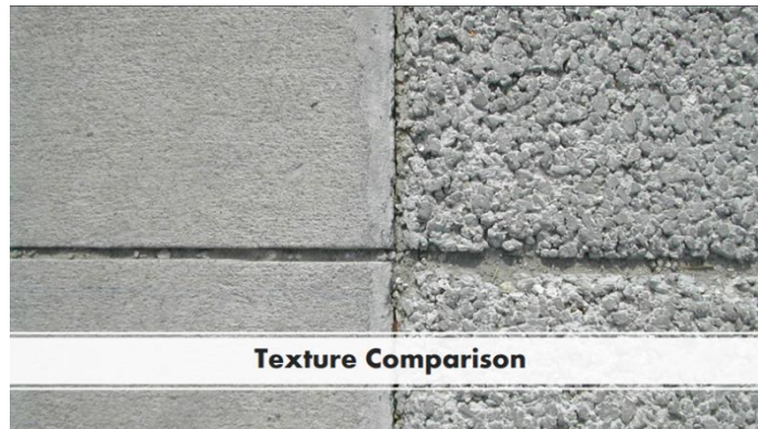
Gambar 1. Perbandingan tekstur beton konvensional dan beton porous (Sumber: Florida Concrete & Products Association, 2019)
