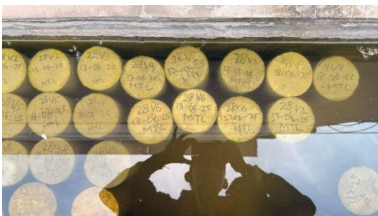
Gambar 3 Water Curing Beton
