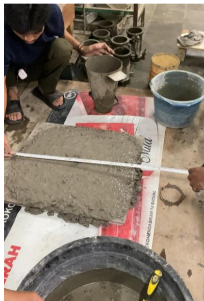
Gambar 1 Pengujian Slump-Flow test
