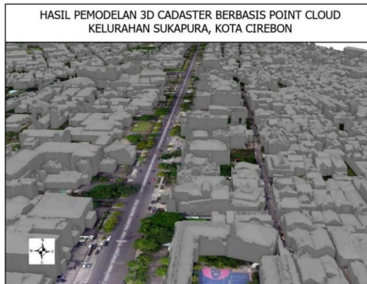
Gambar 2. Hasil model 3D berbasis Point Cloud
