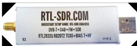
**Gambar 1. RTL- SDR Realtek RTL2832U tuner Rafael micro R820T2**
