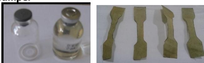
**Gambar 1. Sampel Minyak Gas to Liquid dan Kraft Paper**
